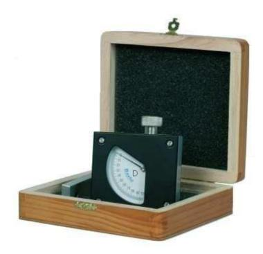
To determine the Shore D scale hardness of specimens and articles of hard rubber and its derivatives, according to UNE EN ISO 868, ISO 48-9, ISO 7619, DIN 53505 AND ASTM D 2240-15. Used in the following types of materials: Hard thermoplastic, hard rubber and plastic high hardness, plexiglass, polystyrene, sheet vinyl, cellulose acetate, thermostatic and laminated formica, etc.
