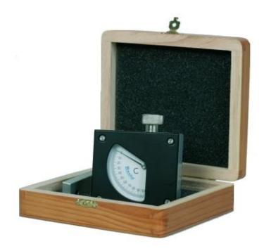
To determine the Shore A scale hardness of probes and medium hardness articles according to ASTM D 2240 standard. Used in the following types of materials: Medium-hard rubbers and plastics. Plaster, gypsum. Others.
