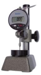
Baxlo Digital Precision Series thickness gauges combines the easy handling of our dial thickness gauges with the multiple functions provided by digital technology.
